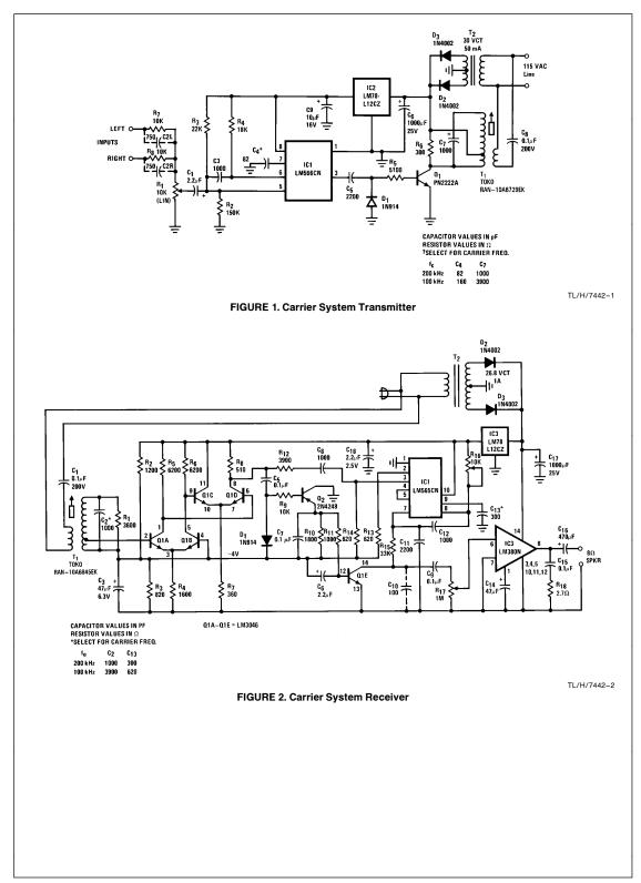
$C_{10}=100\ \text{pF}$  will reduce the carrier level fed to the power amplifier. Even though the listener cannot hear the carrier, the audio amplifier could overload due to carrier signal power.
